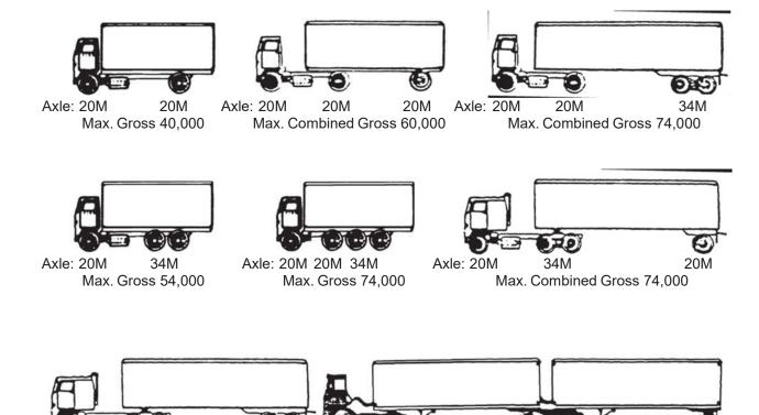
The maximum weight of 20,000 pounds can rarely be placed on the front axle so maximum gross weights shown above would frequently be excessive. Bridge laws will also limit weight according to axle spacing.
